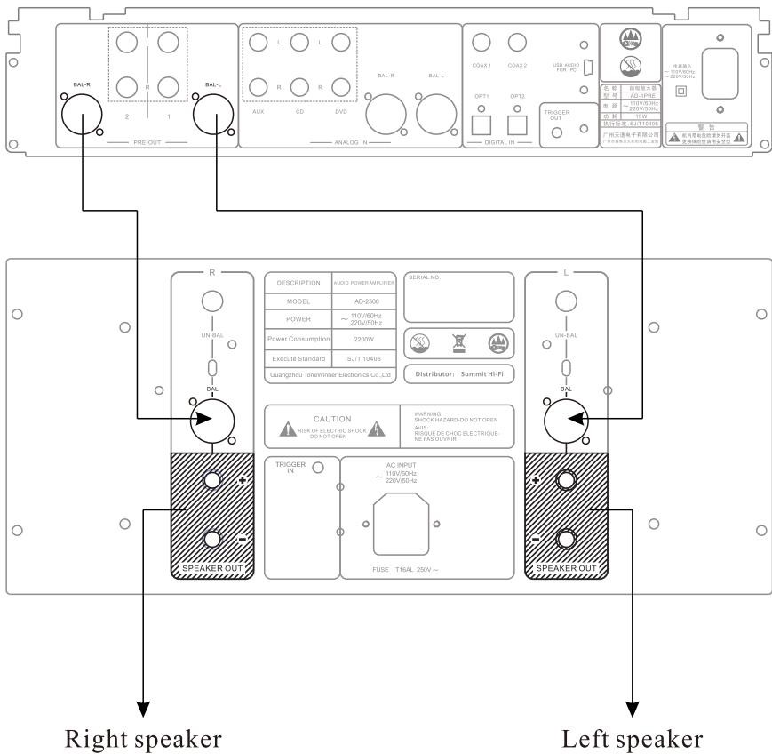
Remark: Should select balance signal on signal channel selection switch.
