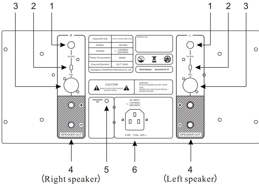
1. Analog signal input port: Signal input port, for connecting with output port of preamp.
